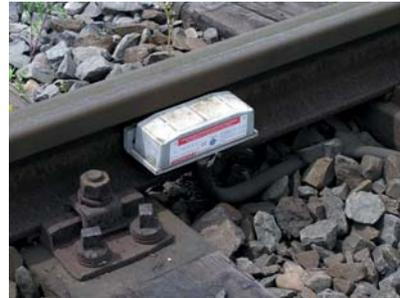
The measured values resulting from gravity marshalling across the topology of the train formation facility (ZBA) are recorded continuously via connected track switching equipment (dual rail switches), radar equipment, light grids, light barriers, wheel load measurement and weather sensors. Time measurement is taken with accuracy greater than 50  $\mu$ s.
