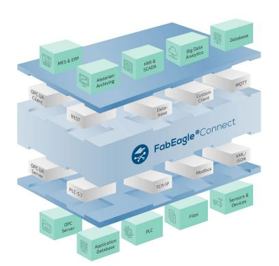
FabEagle®Connect can be used to realize the interface solution on various platforms. Central server are used for the factorywide interface integration. Windows-based IoT gateways and edge devices are also supported for the closest implementation to the machine.
